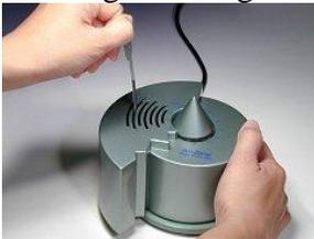
A special steel element cleaning tool has been included with your unit. It can be used to push any dirt out of the elements. The ozone generator can also be set to its highest level for 30 minutes to burn off any accumulated dirt buildup.
